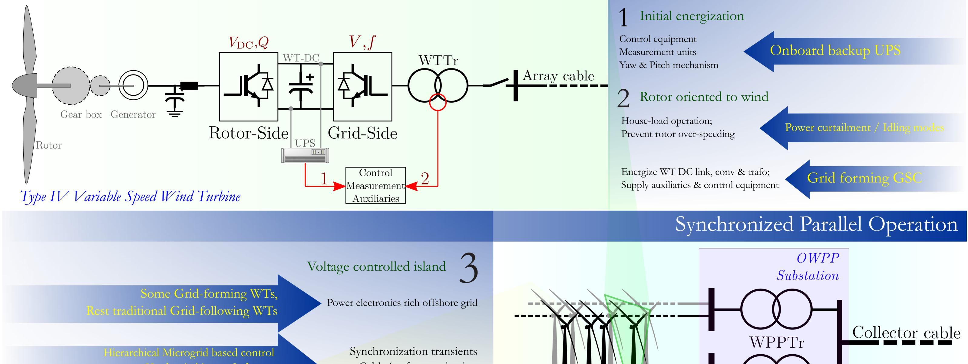
Hard switching vs Soft start PIR, PoWS, Smart energize Cable/trafo energization SOV, TOV, SFO, TRV
